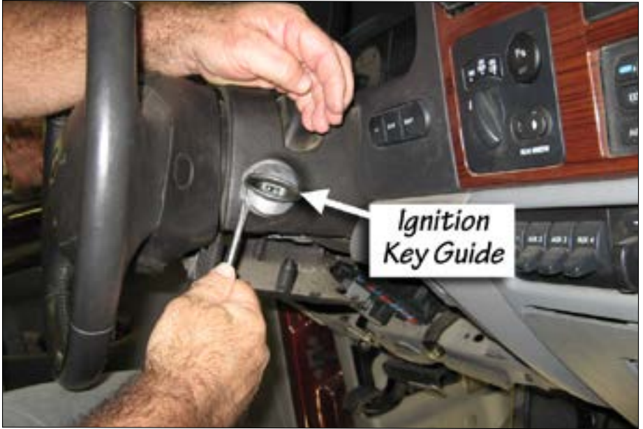
Figure 21 Remove Plastic Ignition Key Guide
