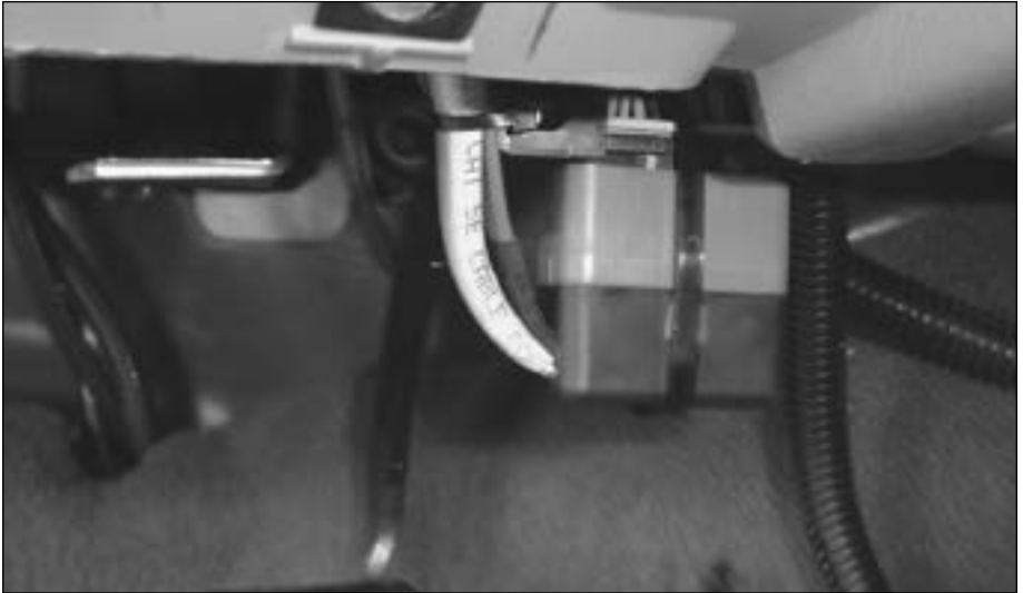
Figure 9: OBDII interface cable
