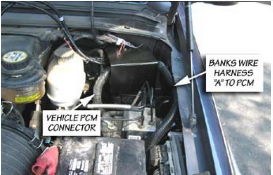
Figure 4: Six-Gun/EconoMind installed on the fuse box on 2005-07 model-year vehicles
