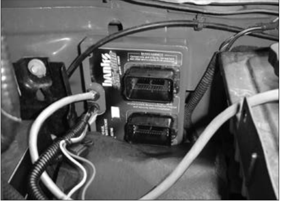
Figure 4: Six-Gun/EconoMind installed on the fuse box on 2005-07 model-year vehicles
