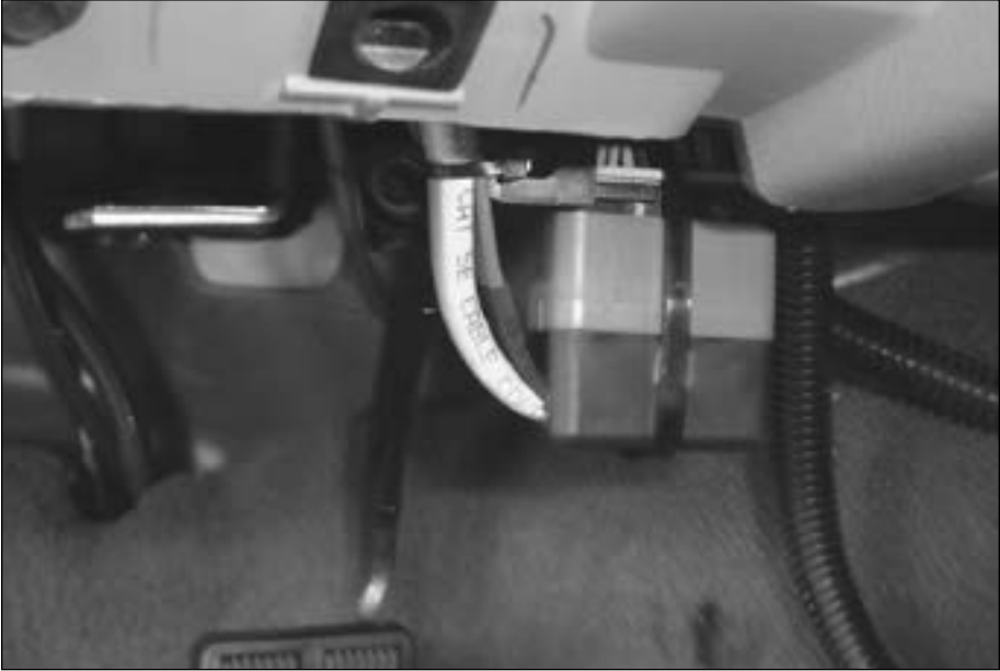
Figure 19 Brake Position Sensor location under dash
